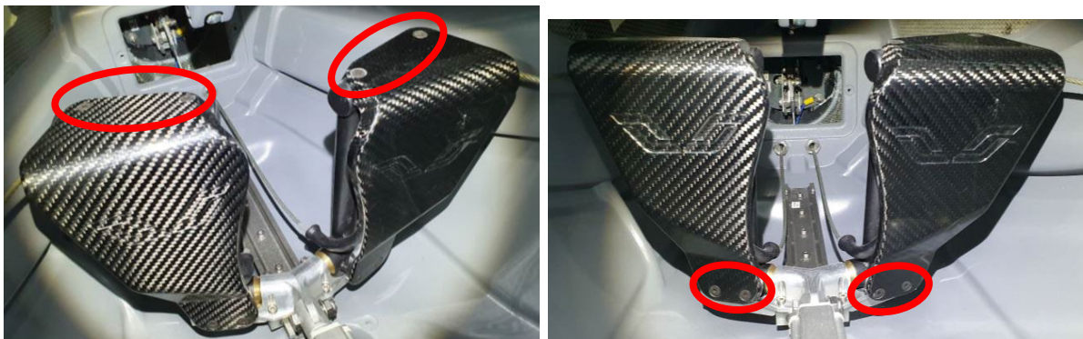
Figure 1: Countersink cap screw locations on footplates (Type 2 shown, similar locations on Type 1)
