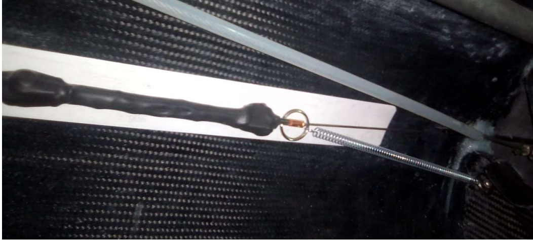
Figure 1: Spring assembly fastening onto tailwheel cable between bulkhead B8 and bulkhead B9
