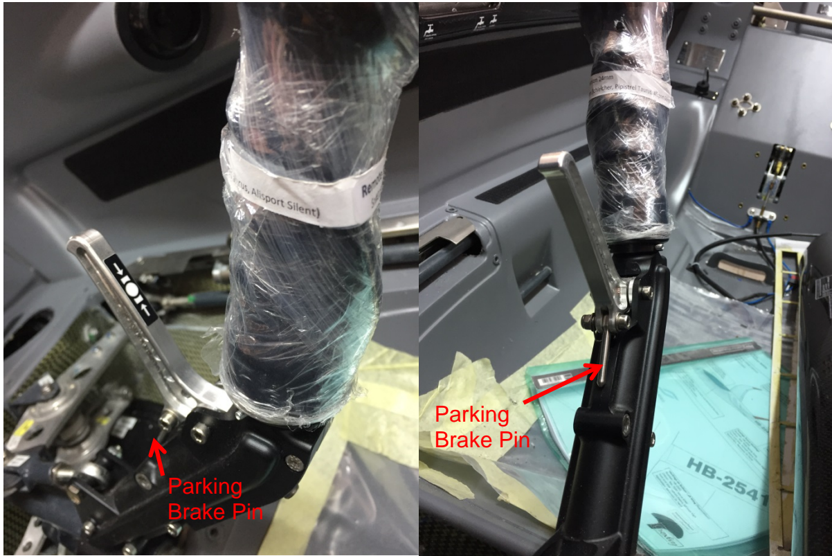
Figure 2: Parking brake pin on the wheel brake lever
