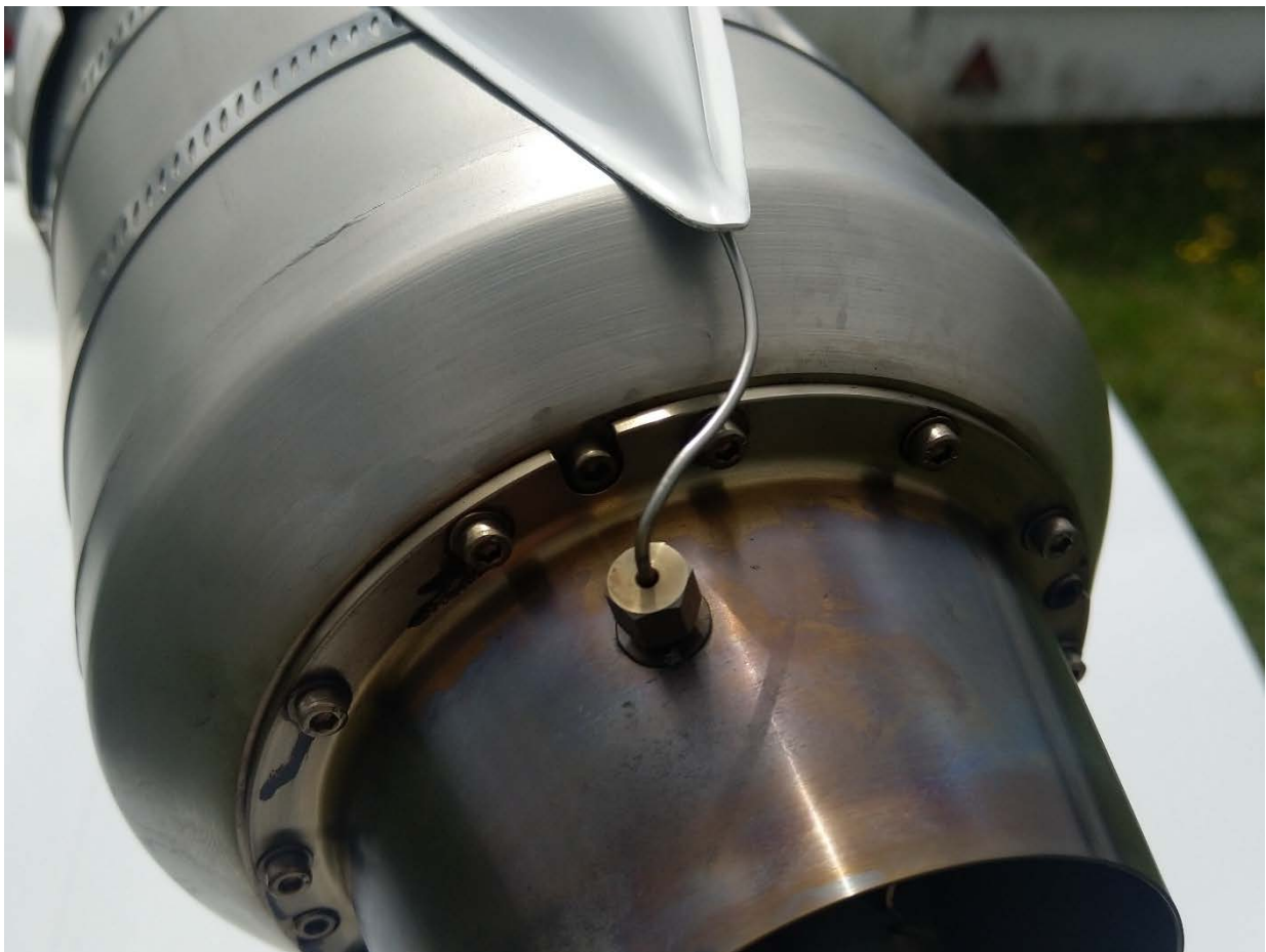
Figure 5-3: Sensor wire routing
